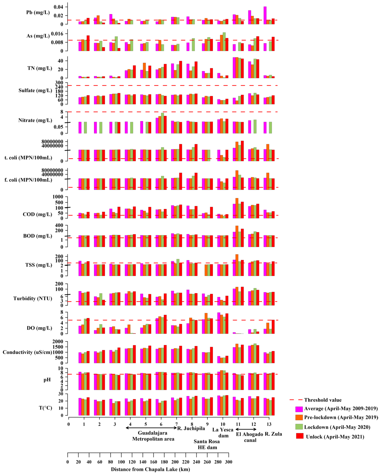
Fig. 2 Levels of 15 water quality parameters in the Santiago River at each sampling location during the pre-lockdown, lockdown, unlock, and 2009–2019 periods
