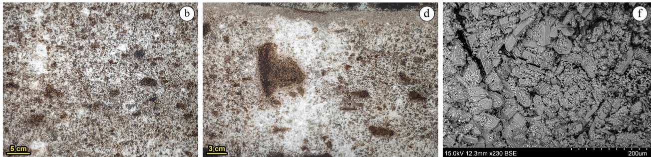
Fig. 5 Sulfate efflorescences with their macroscopic features (a–d) and microscopic texture observed at the SEM-BSE (e–f)
