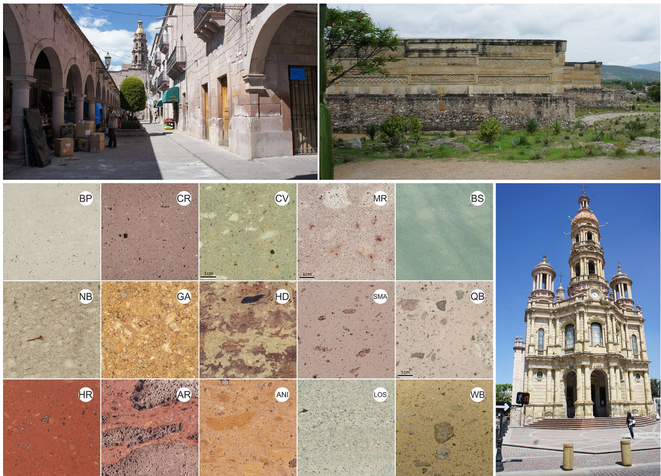
Fig. 1 Volcanic tuffs in building heritage. Top left: the city center of San Miguel el Alto, Mexico; top right: the second century Mitla Pyramids, Mexico; bottom right: the twentieth century Temple of Saint
