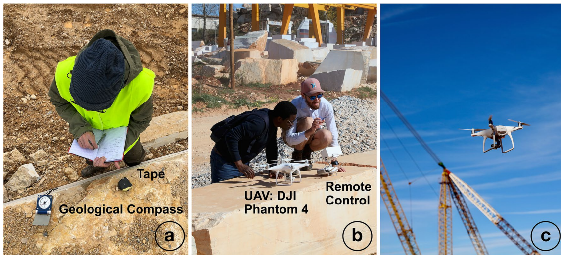
Fig. 9 Data collection by (a) traditional joint survey, using a geological compass and measuring tape. (b) All-in-one UAV: DJI Phantom 4 with remote control. (c) UAV during photogrammetric survey
