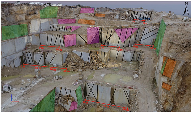
Fig. 18 North facing view of all mining levels with the identified vertical main joint sets. The orange surfaces indicating the NW–SE joint set, the purple surfaces the NE–SW joint set and the green surfaces the NNE–SSW joint set
