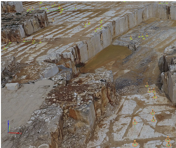
Fig. 10 Point clouds were used to identify the orientation of joints and the joint spacing. In this case, joint traces are visible after rain wetting
