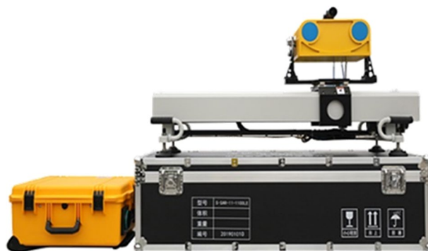
Fig. 4 S-SAR slope monitoring radar
