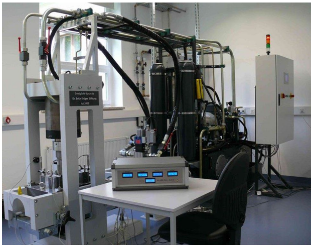
Fig. 2 Big shear box device at the rock mechanical laboratory at TU Bergakademie Freiberg (Konietzky et al. 2012)
