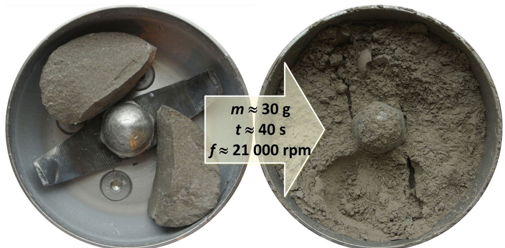
Fig. 2 A photograph of a dolomite sample before comminution (left) and after comminution (right) performed with the GPR analyzer
