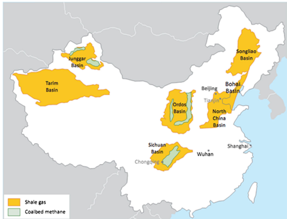
Fig. 1 Overview of shale and tight gas as well as coalbed methane reservoirs in China (Source: World Energy Outlook 2012). The studies presented in this Thematic Issues are dealing with several reservoirs: the Ordos Basin (Liu et al. 2015b), Sichuan Basin (Lu et al. 2015), Songliao Basin (Liu et al. 2015c)
