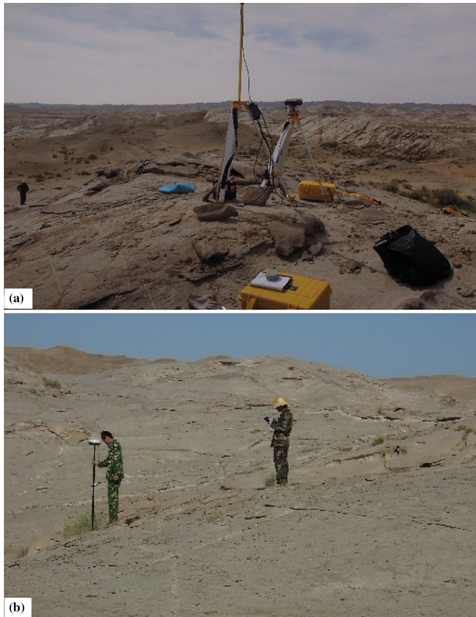
Fig. 2 Measurement of discontinuity in study site by GPS-RTK. a Base station. b Mobile station
