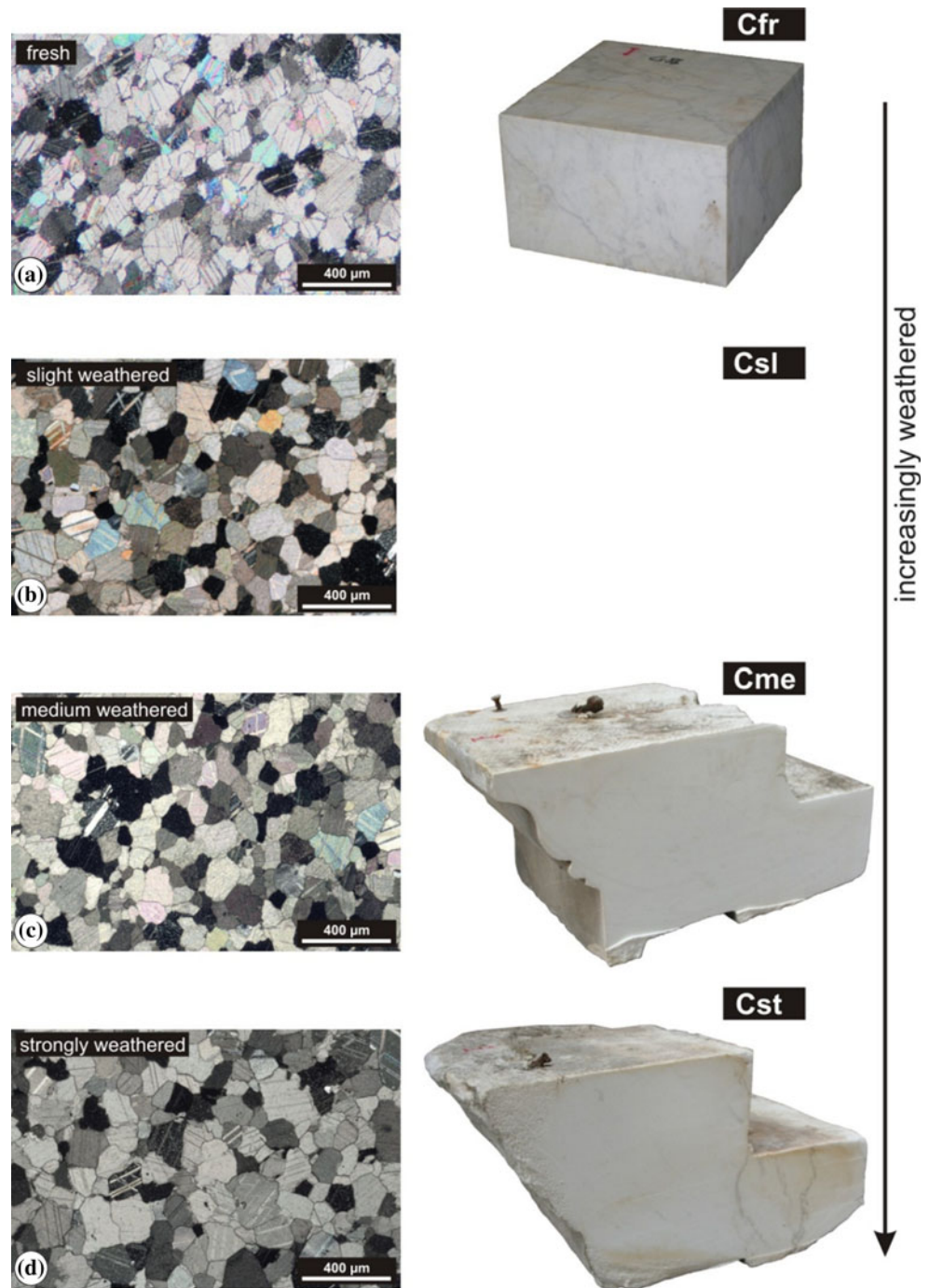
Fig. 4 Investigated samples of Carrara marble: weathered specimens from the Marble Palace in Potsdam and a fresh reference sample from the quarry near Gioia (Italy)
