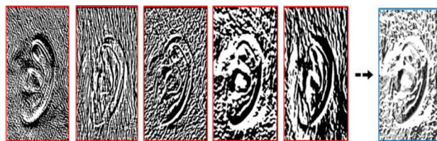
Fig. 4 Binary hashing process: images with red border are feature maps produced by the convolution layer, the rightmost image with the blue border is the result of fusing these feature maps (color figure online)
