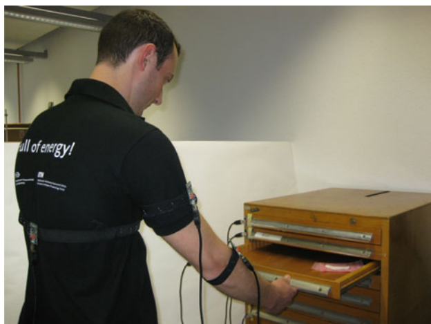
Fig. 9 Setup: 13 drawers equipped with ambient ContextCells (trainer) and 3 wearable ContextCells (learner) on body
