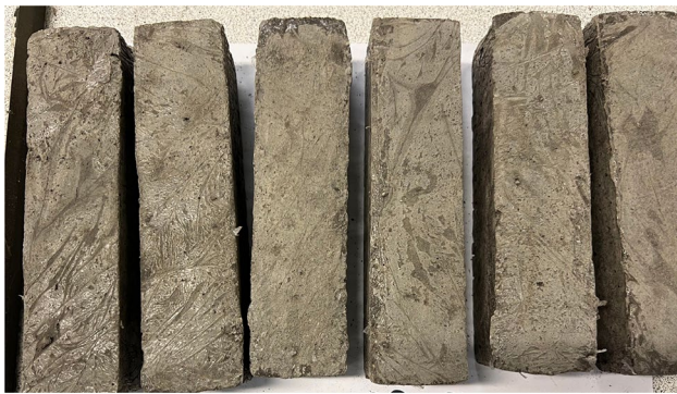
Fig. 3 Prism mortar samples after demoulding
