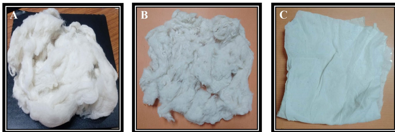
Fig. 4 Bio-scoured non-spinnable cotton ( A short staple cotton; B cotton Linters; C non-woven cotton fabric)
