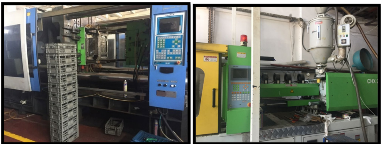
Fig. 10 Industrial manufacturing of crates and table legs from WPC compounds by using injection molding process
