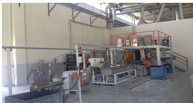
Fig. 2 Process line of industrial manufacturing of WPC compounds
