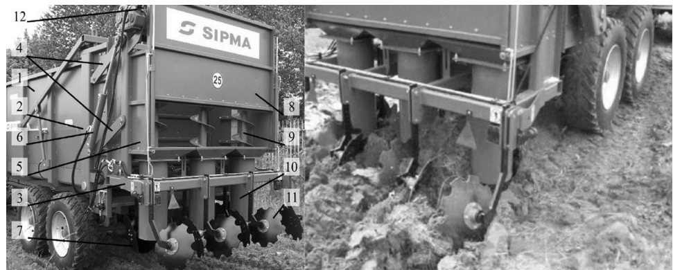
Fig. 3 Prototype of the device for subsurface application of loose organic and mineral fertilizers manufactured by SIPMA S.A.: 1—trailer, 2—base frame, 3—beam, 4—arms, 5—loading chamber, 6—hydraulic cylinder, 7—disc coulters, 8—flap, 9—screw conveyor, 10—cylindrical housing of screw conveyor, 11—ridging plough, 12—hydraulic engine
