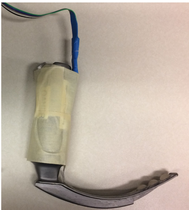
Fig. 2 GlideScope Titanium T-MAC blade with dome-shaped plastic pucks glued to FlexiForce sensors, as recommended by the manufacturer, Tekscan Inc., Boston, MA, USA
