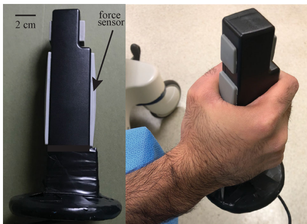
Fig. 1 Dynamometer. The left panel shows the dynamometer with the metal disc attached at the inferior end to obtain a total weight of 1.2 kg. The right panel shows the holding position
