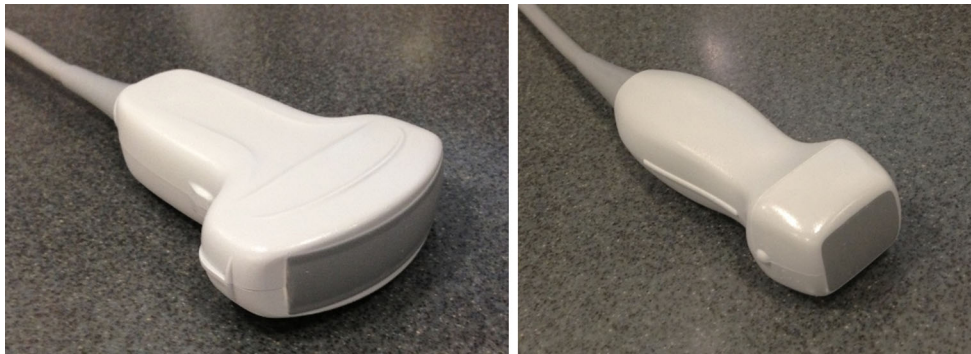
Fig. 2 Transducers suitable for the Focused Assessment with Sonography in Trauma (FAST) exam: the curvilinear (left) and phased array (right) probes each offer excellent penetration into the
