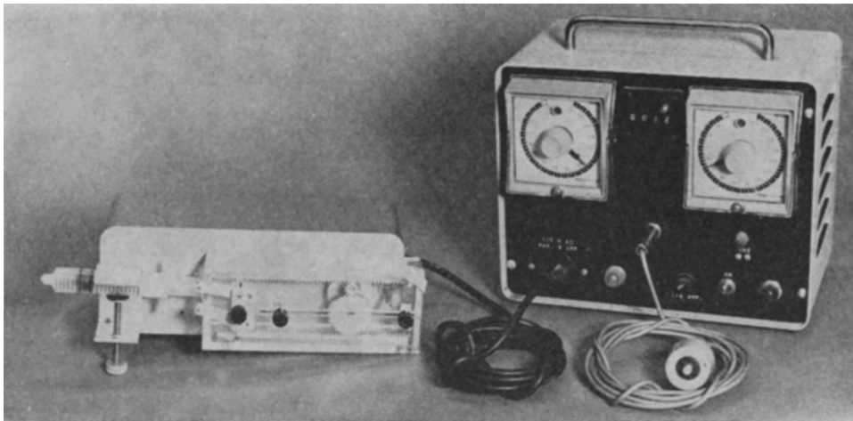
Figure The complete apparatus. Left: The motor syringe. Right: The switchbox. Top array, lft to rt.: Timer A, counter, timer z. The dark circles at 12 o'clock on timer dials are pilot lights. Middle array, l/t. to rt.: push-button lead, beeper light. Bottom array, lft. to ft.: motor syringe socket, motor syringe circuit pilot light, fuse, on-off switch, switch-box circuit pilot light. Wiring diagram may be obtained by applying to the manufacturer-Canadian Algor Ltd, 159 Albert Street, London, Canada. Reproduced with permission from: Keeri-Szanto M. Apparatus for demand analgesia. Can Anaesth Soc J 1971; 18: 581-2
