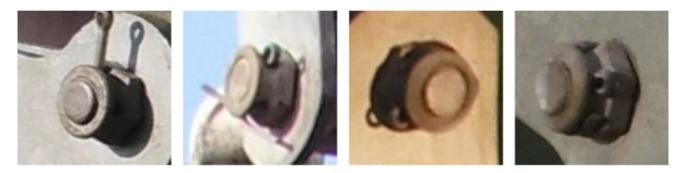
Fig. 4 Exemplary images of the *safetypin* component type from the  $DS_{Pi}$  dataset. The defective *safetypins* (two to the left) are not completely bent, while the intact ones (two to the right) are completely bent and consequently prevent slipping out
