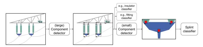
Fig. 5 Structure of our multistage power line component detection and classification pipeline for high-resolution images
