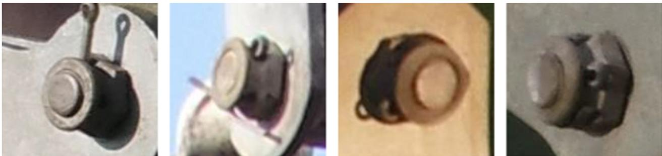
**Fig. 4** Exemplary images of the *safetypin* component type from the  $DS_{Pi}$  dataset. The defective *safetypins* (two to the left) are not completely bent, while the intact ones (two to the right) are completely bent and consequently prevent slipping out
