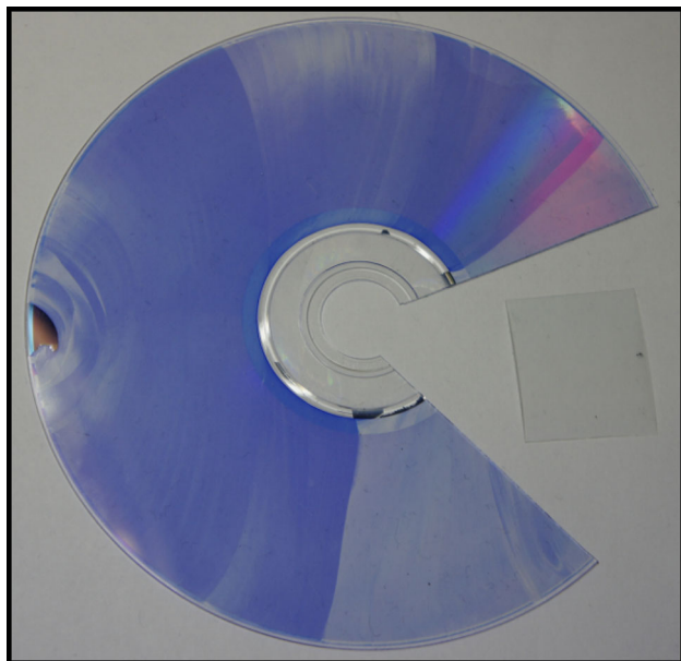
Fig. 3 DVD as grating source for spectrometer
