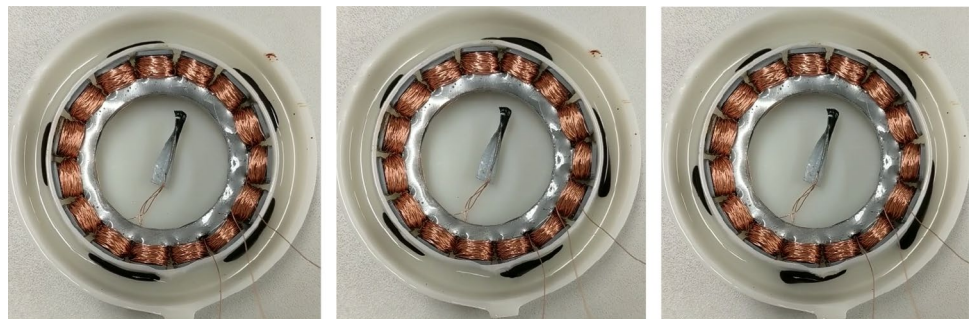
Fig. 6 Picture of the first Ferrowheel concept that consists of no solid moveable components. A ferrofluid droplet, contained in a basin together with a suitable secondary liquid, is accelerated through a 3-phase AC of the stator
