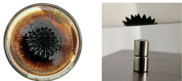
Fig. 2 Pictures of the Rosensweig effect of ferrofluid, left with the ambient air as secondary fluid and in the right, with isopropanol. Underneath the petri dish left is a permanent magnet placed so that the magnetic field is perpendicular to the ferrofluid. The structure of peaks and valleys is visible
