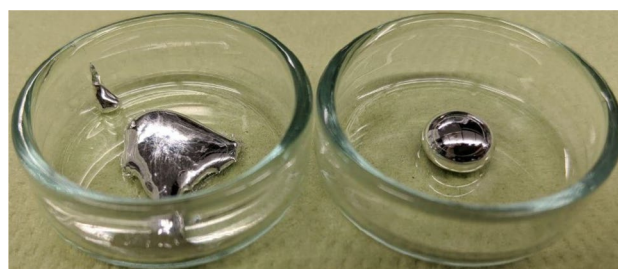
Fig. 3 On the left is oxidized Galinstan, with a clearly visible skin layer appearing above one ppm oxygen content. On the right is a typical spherical liquid Galinstan droplet, hereafter reduction of the oxygen layer with hydrochloric acid
