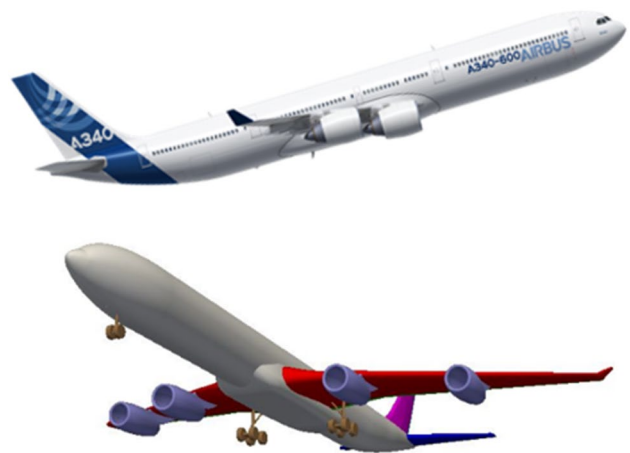
Fig. 12 The A340-600 in clean configuration (top) and in IAC configuration (bottom) [11]
