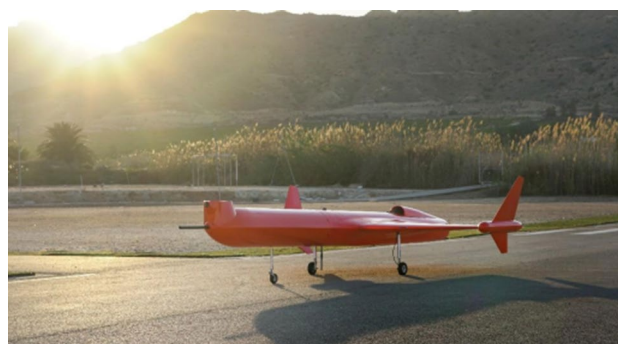
Fig. 5 RLV demonstrator (RLVD) during taxi testing [7]
