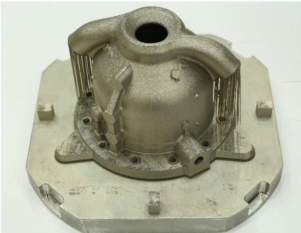
Fig. 15 Combustion chamber of the newly designed aerospike engine after manufacturing via LPBF
