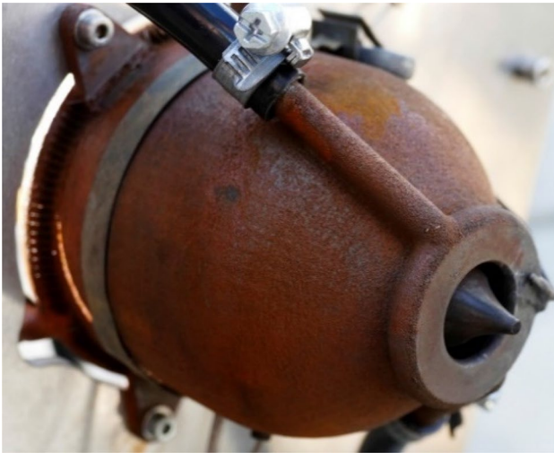
Fig. 6 Corrosion on the outside of the 2019 aerospike demonstrator made of X40CrMoV5-1
