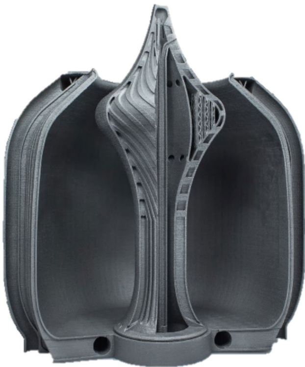
Fig. 2 Additively manufactured cutaway model of the manufacturing demonstrator [5]
