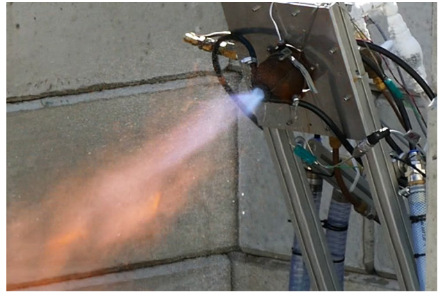
Fig. 3 Hot fire test of the 500 N aerospike engine
