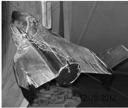
Fig. 25 Oil visualization for model 1212 \alpha=27.5^\circ , \beta=20^\circ , and V=20 m/s
