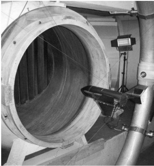
Fig. 9 The experimental model hanged in the wind tunnel for the directional cases
