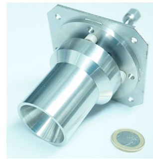
Fig. 2 Thruster prototype with a 25^\circ nozzle
