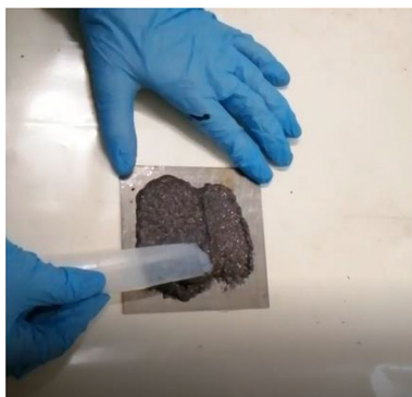
Fig. 4 Application of TPS paste on a steel substrate
