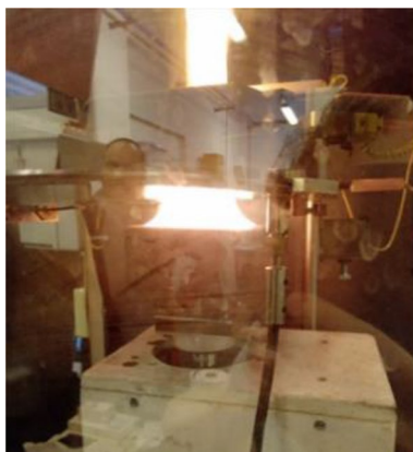
Fig. 6 Cone calorimeter test
