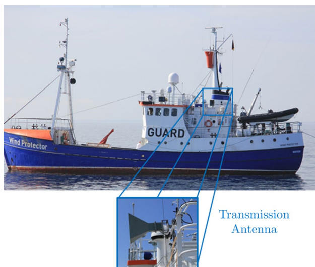
Fig. 9 Jammer installation showing a horn antenna and a small helix antenna
