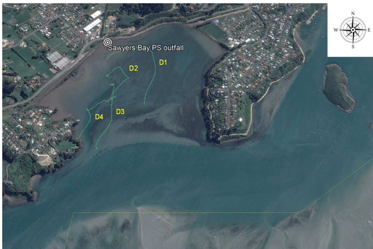
Fig. 4 Drogue tracks (shown as green lines) in Sawyers Bay. N.B. All drogues were released at inshore sites and travelled towards the mouth of the bay
