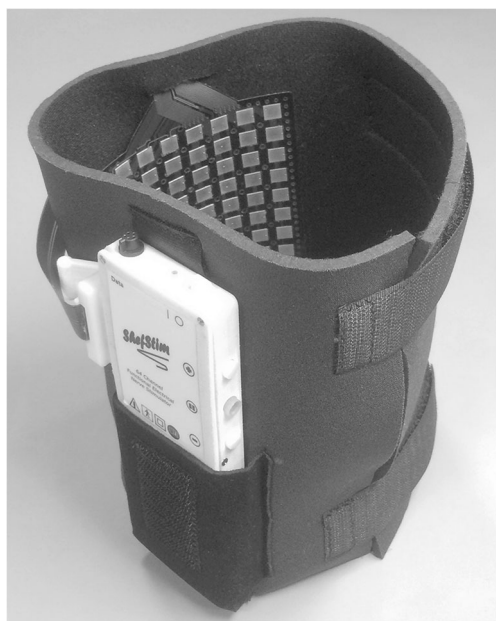
Fig. 1 Sensory barrage stimulator (ShefStim-SBS 64-independent channel stimulator)
