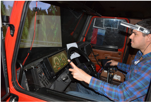
Fig. 1 The truck driving simulator used in the experiment, including the head-mounted PDT
