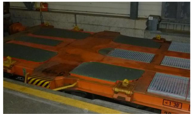
Fig. 8 Swiss Split wagon with inlay elements (Wascosa)
