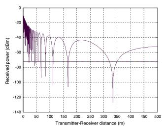
Fig. 4 Received power at 5.9 GHz, along the LX to vehicle radio link
