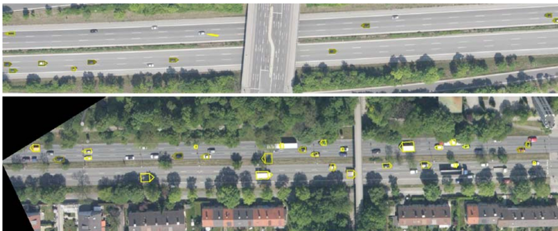
Fig. 5 Examples for vehicle detection on motorways ( upper image , A96 exit Munich–Blumenau, clipped nadir exposure) and in the city ( lower image , Munich “Mittlerer Ring”, clipped side-look-left
