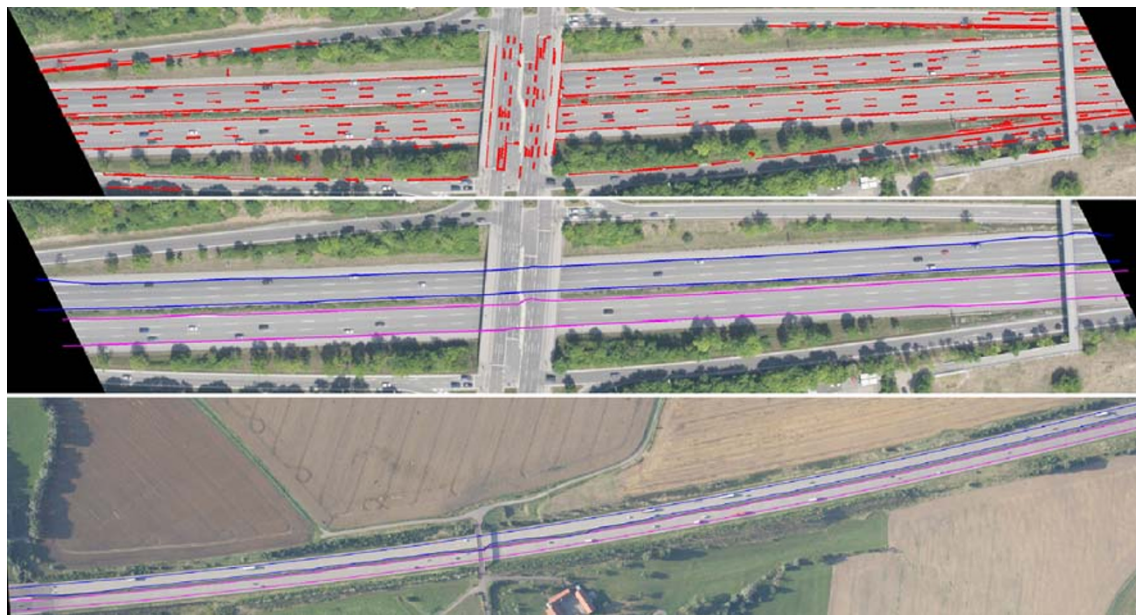
Fig. 3 Examples for road extraction (clipping from nadir images). Upper panel shows line detections at a flight height of 1,000 m, middle panel shows the resulting road area after smoothing/gap filling
