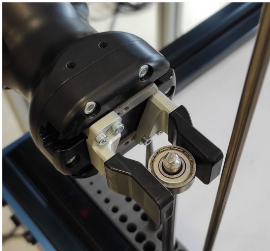
Fig. 10 Assembly operation of a bearing on an 8 mm shaft with the cobot using CSM
