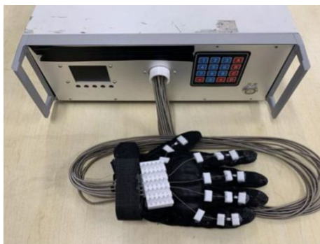
Fig. 7 Hand soft rehabilitation module: hand soft rehabilitation gloves and hand soft rehabilitation control box
