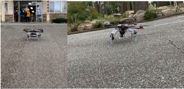
Fig. 12 The quadcopter landing experiment (10° slope)
