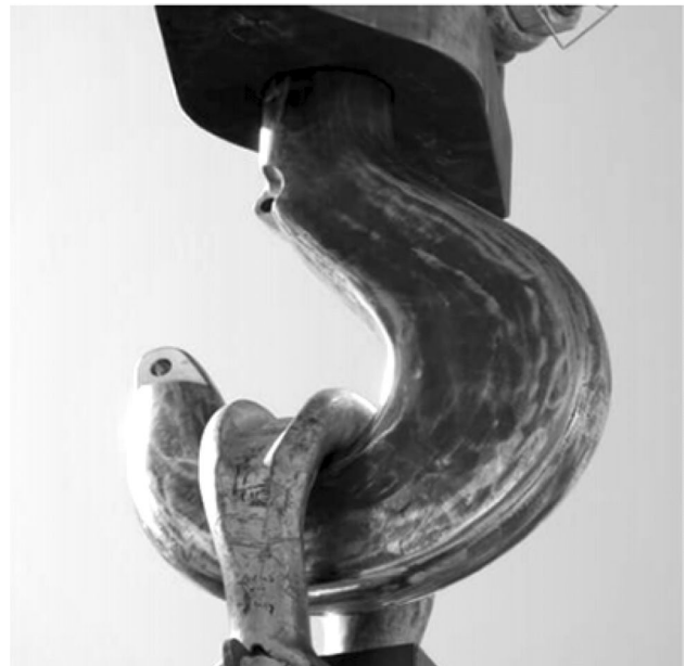
Fig. 17 HUISMAN'S 3D printed crane hook [60]
