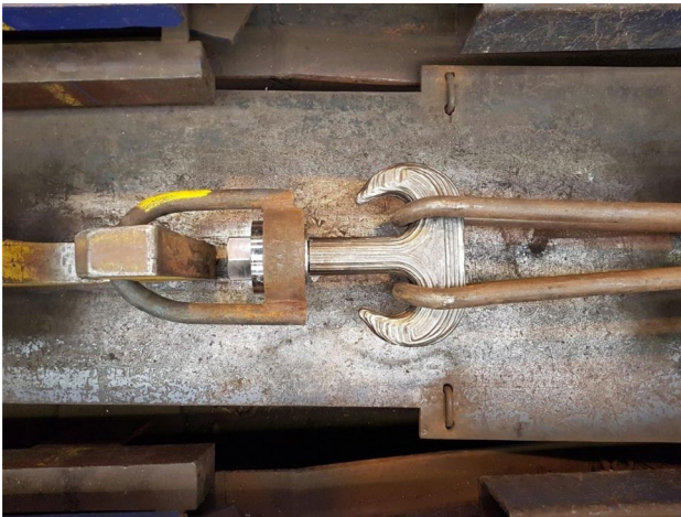
Fig. 16 HUISMAN'S 3D printed WAAM hook [59, 60]
