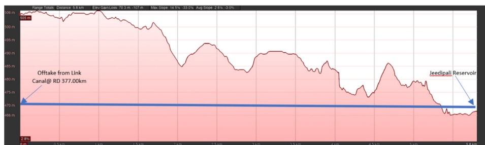
b Longitudinal section of the link canal connecting the A-P ILR link canal to the Jeedipalli reservoir
