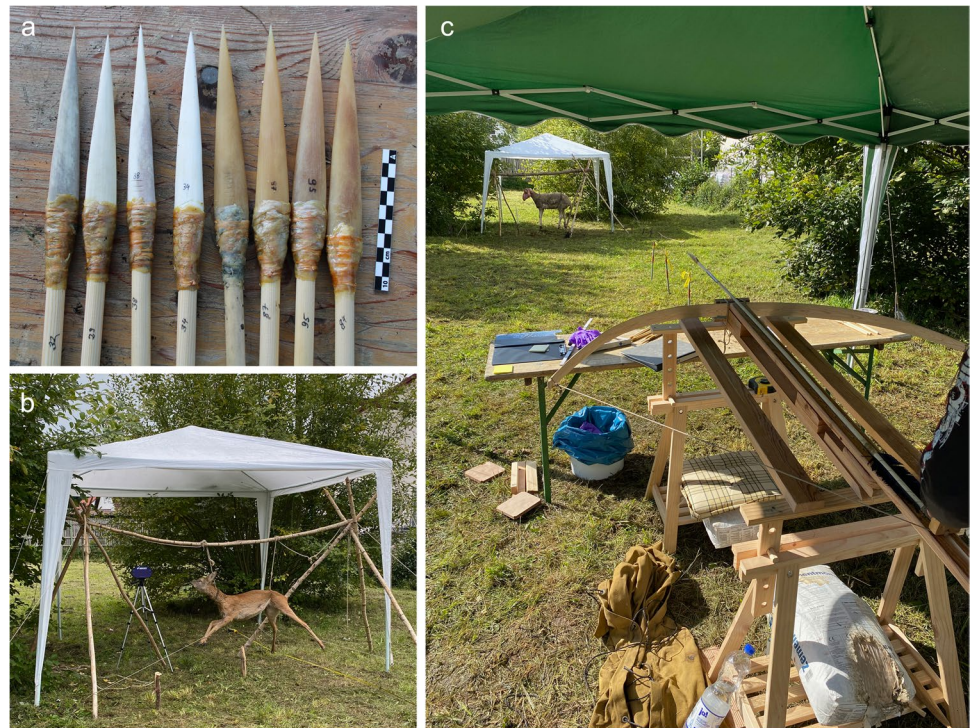
Fig. 1 The shooting experiment: (a) selected bone and antler projectile replicas used in the shooting; (b) target 1 (sub-adult roe deer); (c) the calibrated crossbow and target 2 (adult sheep)
