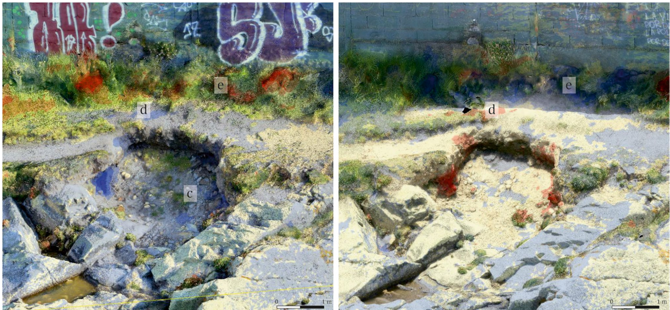
Fig. 15 Detail of the changes produced in Sector 2, using as reference the model C1 (left) and C2 (right). Areas with loose of material (c) and (d), area with a gain of material (e). Oblique view from the northwest
