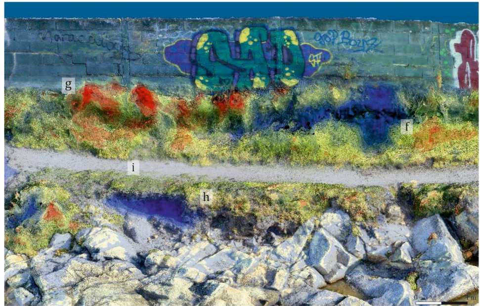
Fig. 16 Detail of the changes produced in Sector 3, using as reference the model C1. Areas with a loose of material ( f ), ( h ) and ( i ); areas with a gain of material ( g ). Frontal view from the north
