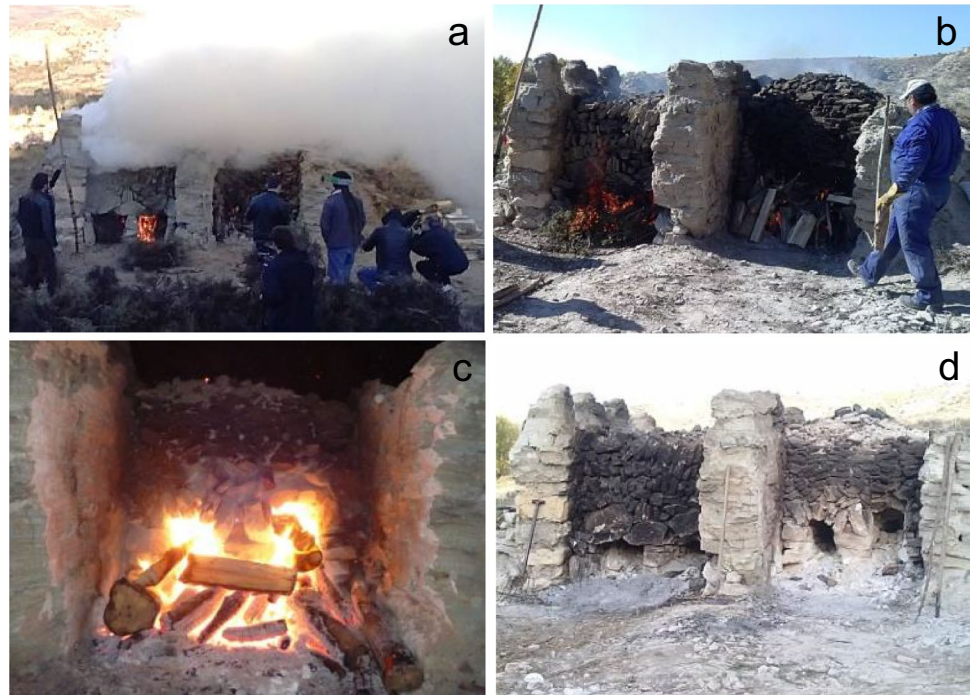
Fig. 10 Experimental gypsum calcination in two traditional kilns performed in 2016 using scrubs (left kiln) or firewood (right kiln): a dense, whitish smoke due to water release is generated during the initial calcination phase; b and c kilns during advanced stages of calcination, reaching a T of up to 1100 °C; and d traditional kilns during the cooling phase
