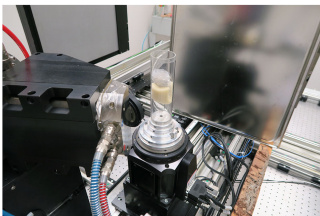
Fig. 6 Amulet fixed inside a Plexiglas tube installed on a rotation stage between the X-ray tube and detector. The detector right behind the stage is covered by steel sheets to reduce the scattering effect. A tin filter cutting-off low-energy photons is mounted onto the X-ray tube head in front of the sample at left. The distance between the tube and detector is minimized to have the maximal possible photon flux within a given magnification
