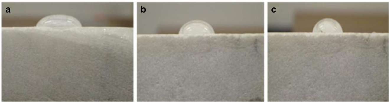
Fig. 11 Drops of distilled water on the surface of the experimental marble samples for static contact angle measurement. a Uncoated sample, b sample coated with pure Paraloid B44, and c sample coated with ZnO nanoparticles/polymer nanocomposites
