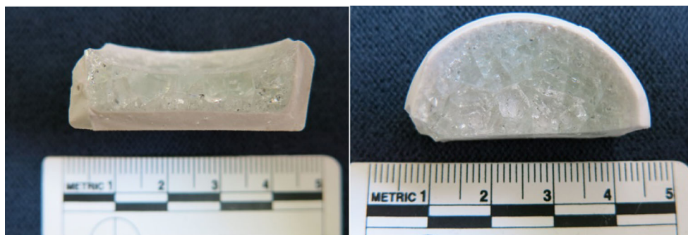
Fig. 3 Glass produced with natron, sand and calcium carbonate melted at 1100 °C for 12 h ( left , glass in section; right , top view of glass in crucible)
