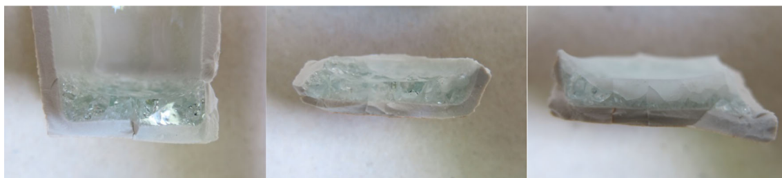
Fig. 2 Batches 1–3 (left to right) show experimental melts made with natron, sand and calcium carbonate melted at 1300 °C for 12 h. Only batch 1 (left) shows a batch-free glass
