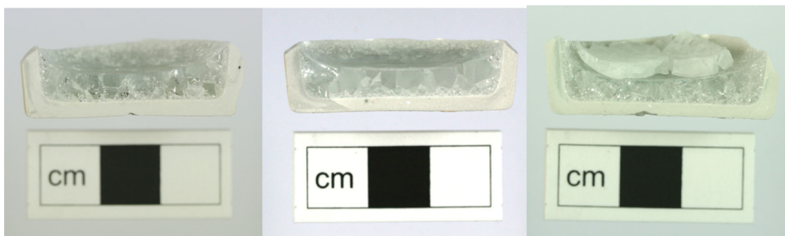
Fig. 4 Model glasses made with sand, calcium carbonate and left to right : sodium chloride, sodium bicarbonate and sodium sulphate ( left ); sodium bicarbonate and sodium chloride ( middle ); and sodium carbonate and sodium sulphate ( right )
