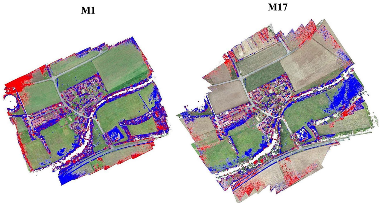
Fig. 6 Areas with detected changes between survey 1 and 2 of M1 and M17 in the Laufer Muehle area ( |d_{M3C2}| \geq 0.25 \text{ m} ; red: elevation increase in survey 2; blue: elevation decrease in survey 2)
