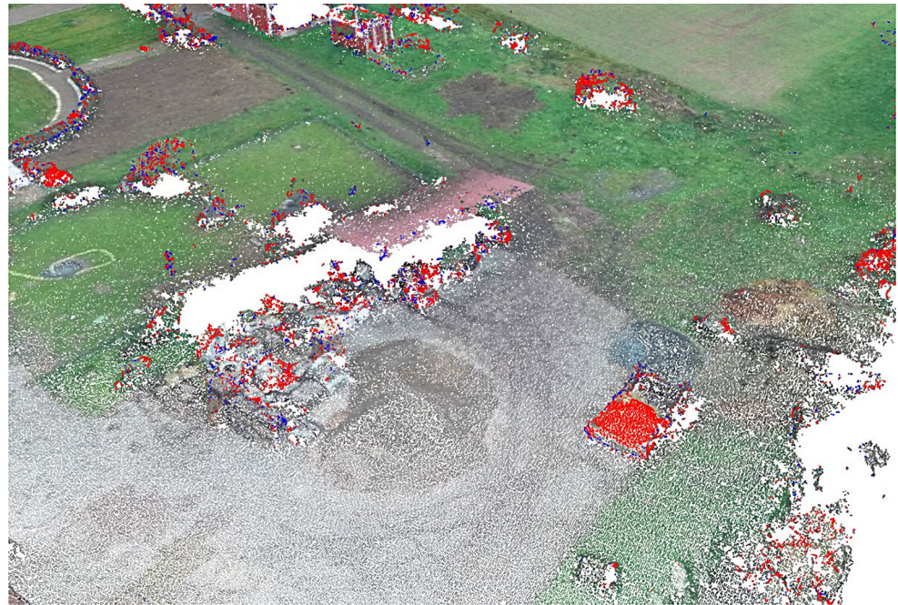
Fig. 9 CD between M1 survey 1 and M17 survey 2 ( |d_{M3C2}| \geq 0.25 \text{ m} ; red: height increase in survey 2; blue: height decrease in survey 2)
