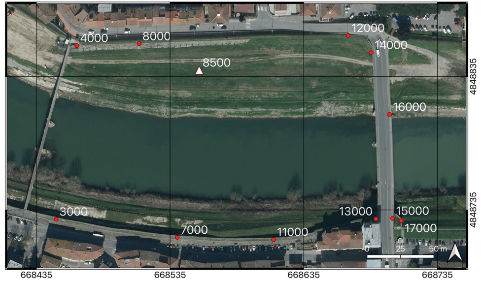
Fig. 11 Orthophoto with control network's vertexes
