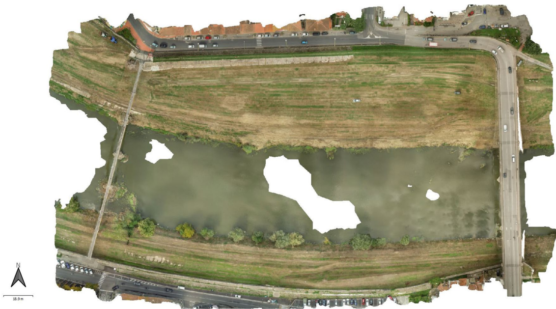
Fig. 18 Raw orthophoto of the surveyed area (300 m in length and 170 m in width)
