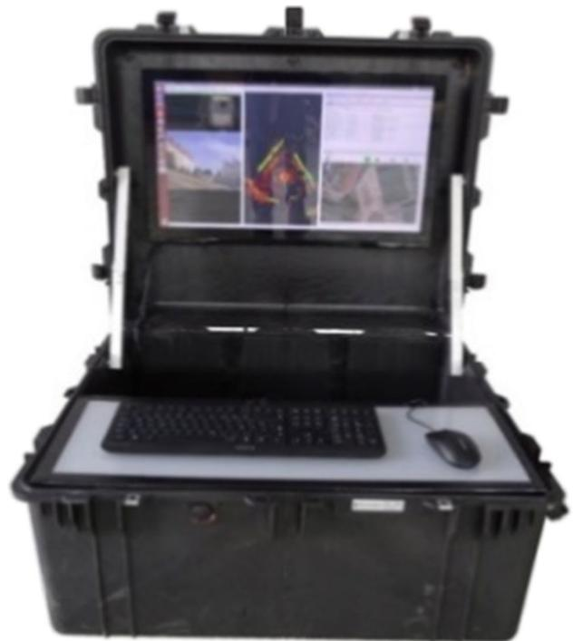
**Fig. 2** ANKommEn—ground control station, source: Batzdorfer, et al. (2018)
