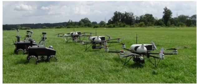
**Fig. 1** ANKommEn data capturing system including UAVs (type: AR200) and UGVs (type: Summit XL Robotnik), source: Batzdorfer et al. (2018)
